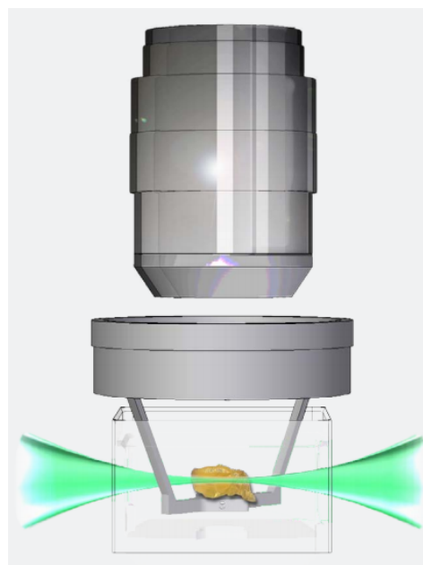
Figure 2.1. Diagram of sample in holder inside reservoir with clearing solution.
