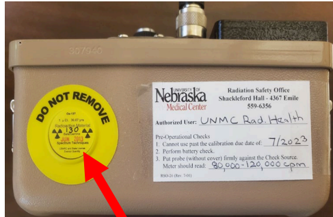
Button Check Source (Typically, Cesium-137)
