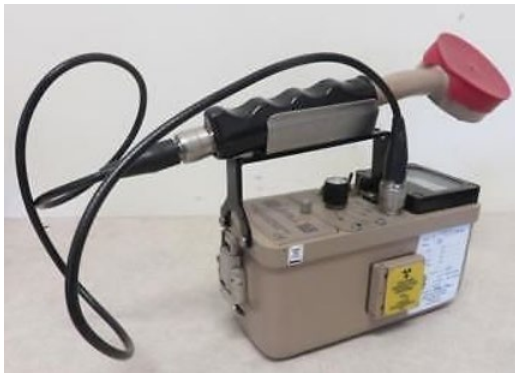
Survey meter with Ludlum 44-9 GM Pancake probe
