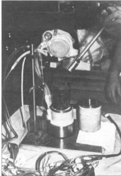
FIG. 4 The NHLI atomic heart. This nuclear-powered heart assist system consisted of two main parts: (1) the blood pump or Model VIII assist pump (top), which is attached via hydraulic drive lines to (2) the thermal converter or nuclear engine (bottom). This photo shows the system being held in an assembly stand during the insertion of the plutonium-238 fuel capsule (center) into the engine prior to implantation. (Source: John C. Norman et al., "An Implantable Nuclear-Fueled Circulatory Support System," Annals of Surgery 176, no. 4 [October 1972]: 497. Reprinted with permission.)
